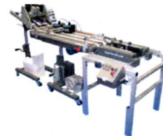
Inline as an accumulator / bundler featuring SmartCount Batch Count Controller
